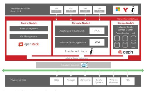
Figure 1. Wind River Titanium Control
